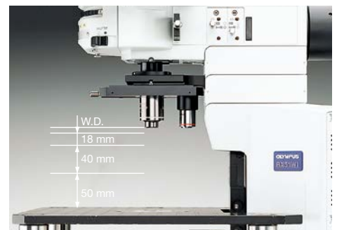
Detaching the condenser assembly and lowering the stage by 50 mm provides maximum clearance
