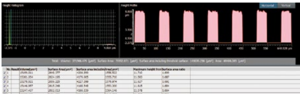
Metal bump / Joint uniformity (Height evaluation) (MPLAPON20XLEXT)
