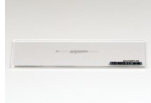
X-Y calibration standard OLS50-CS-XY
