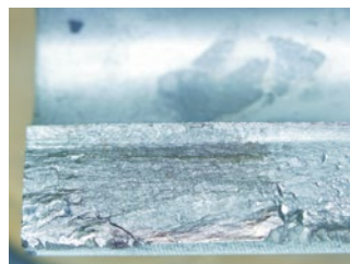
Four-part illumination of surface fracture (metal)
