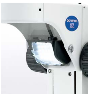
Flexible angle of the LED light source
